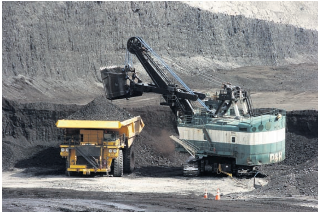
In this April 4, 2013 file photo, a mechanized shovel loads a haul truck that can carry up to 250 tons of coal at the Spring Creek coal mine near Decker, Mont.
